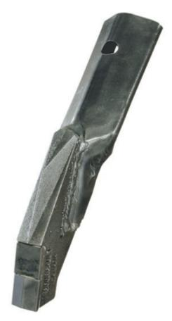
These 1 inch (25 mm) vertical knives are our longest wearing openers. The high chrome cast tip has a double carbide insert that protects the bottom 2 inches (50 mm) of the tip.
