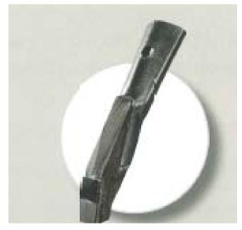
This knife has the same 1" (25mm) tip as the 200-VRT-1011. The high chrome cast tip has a double carbide insert that protects the bottom 2" (50mm) of the tip. Because of the near vertical approach, this opener will pull harder than conventional knives, however it will throw less soil and pull out fewer rocks.
